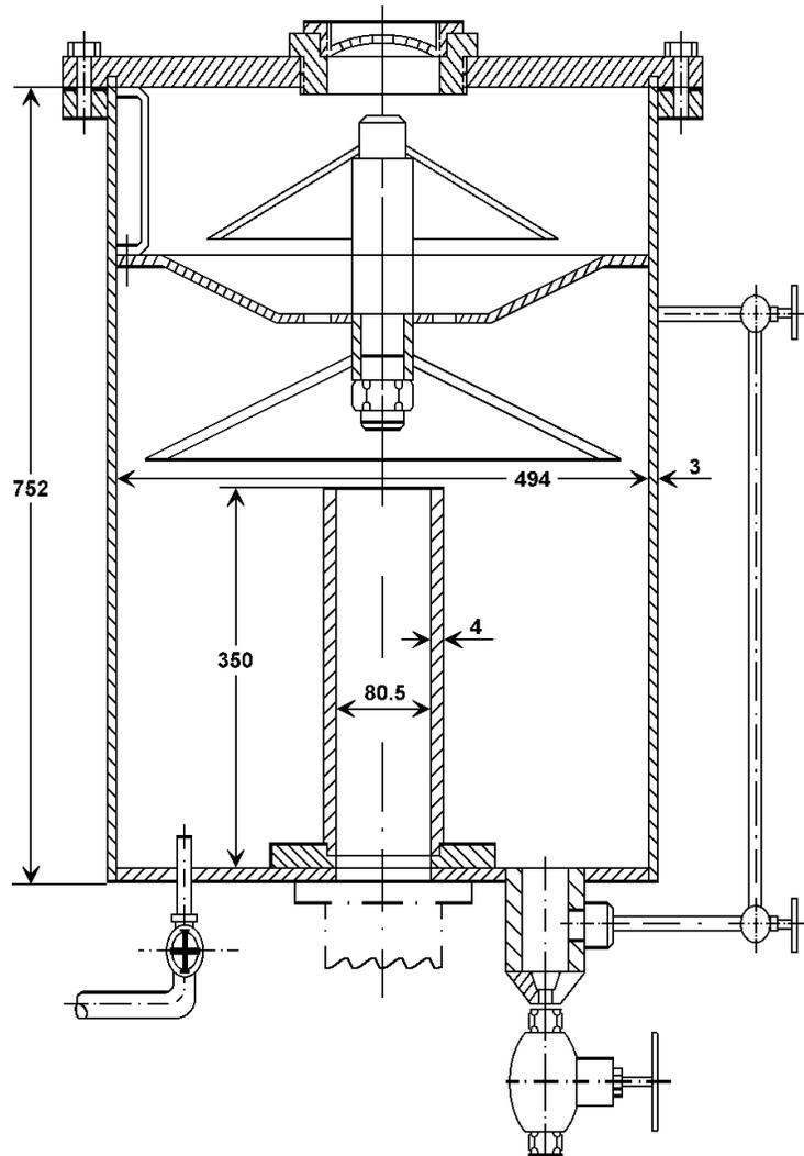
Figure 16. Oil reservoir (Dimensions are in mm).
