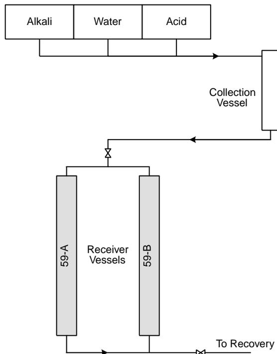
Figure 32. Major components of the chemical-etching process.
