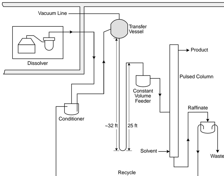
Figure 25. Process equipment related to the criticality accident.
