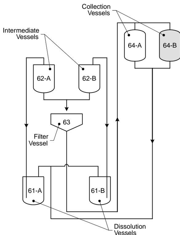
Figure 18. Process vessels and material flow diagram.
