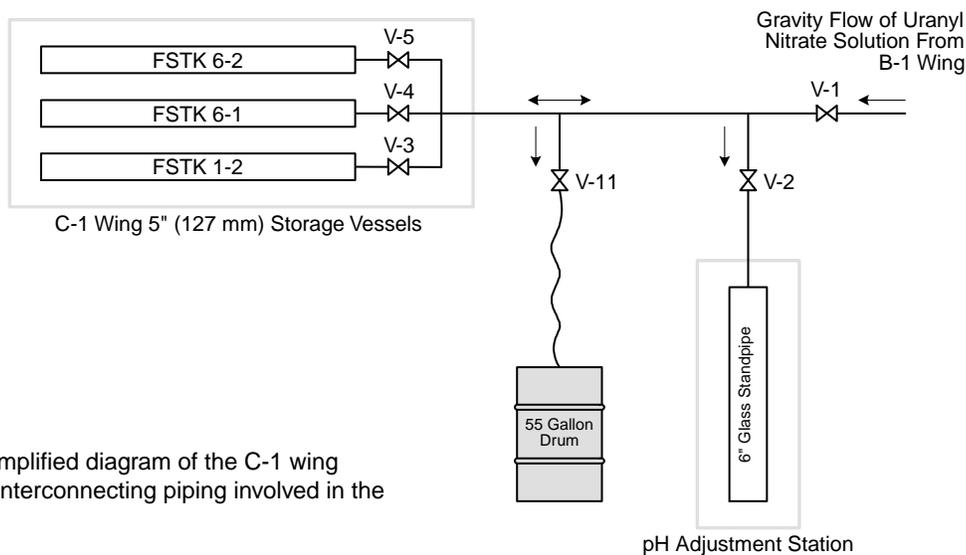
Figure 9. Simplified diagram of the C-1 wing vessels and interconnecting piping involved in the accident.
