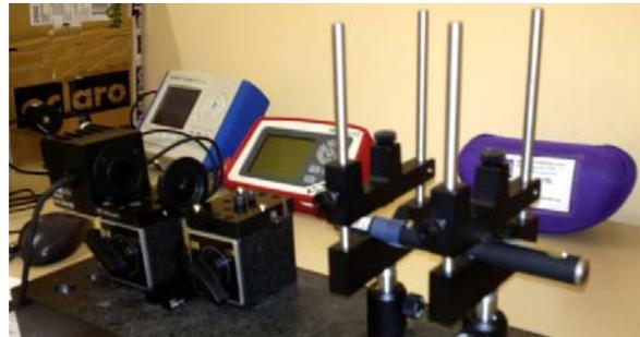
Figure 1 The measurement setup for this work, magnetic optics mounts were used to stabilise the laser pointers and the meters. The variation in form factor of the devices meant that flexible supports were required.
